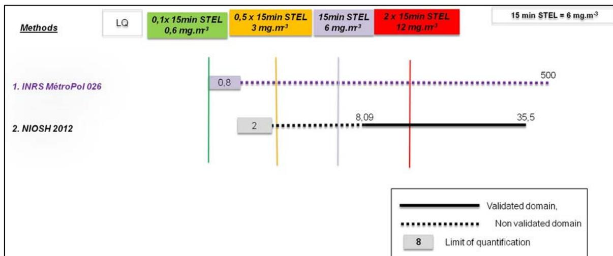
**Figure 1: ranges of validity and limits of quantification for the various compared methods from 0.1 to 2 times the 15min-STEL recommended by the OEL Committee for n-butylamine**
