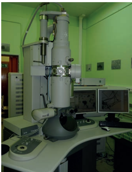
Tecnai spirit transmission electron microscope with biotwin lens configuration operating at 120 kV. Credit CODA-CERVA.
