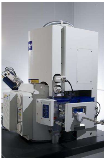
Figure 2 : SEM at LNE (Zeiss ULTRA-Plus equipped of a Field Emission Gun (FEG))
